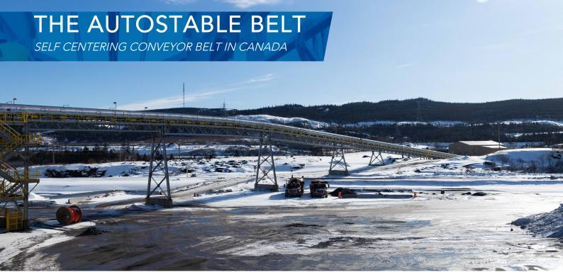
**Autostable** is Sempertrans self-centering conveyor belt, which virtually eliminates lateral movements with a centering force five to eight times higher than that of conventional conveyor belt. "This prevents material loss and all misalignment-related damage to the belt or conveyor system"
