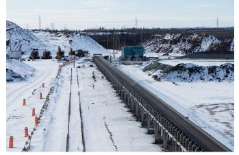
Sempertrans Autostable conveyor belt was the sole solution against the serious mistracking problem the customer was facing. It helped achieve better stability and safety of their conveyor operations, resulting in belt lifetime 3 times longer. Additionally, by increasing the troughing angle, fewer edge damages occurred, particularly in installations with idler adjustment issues.
