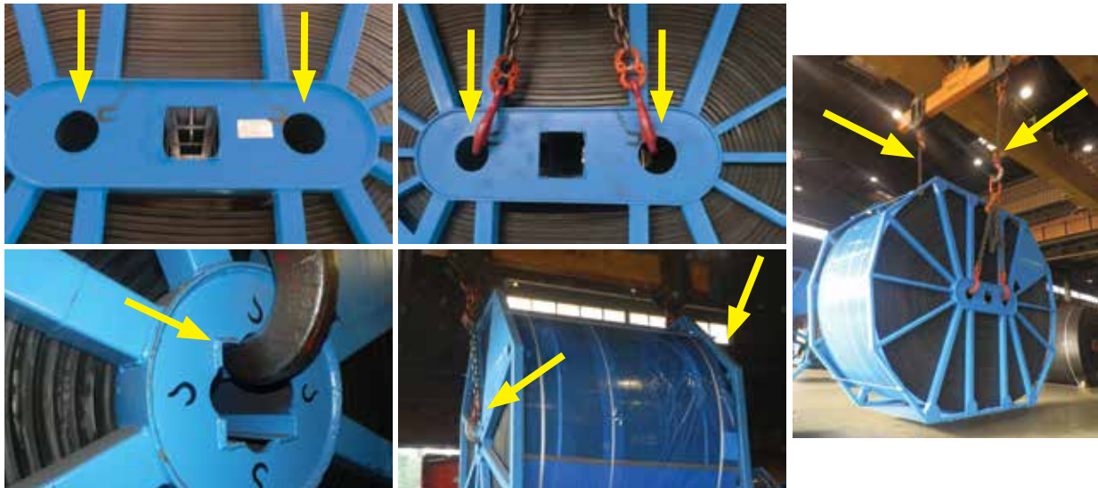
Picture 3: Open ellipse flat rack containers and open steel reels – recommended way of lifting the roll using suitable lifting equipment (a lifting sling is a minimum requirement).
