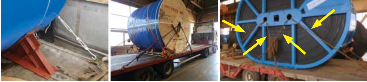
Picture 5: Recommended way of ensuring safety and careful protection of the reels before transportation
