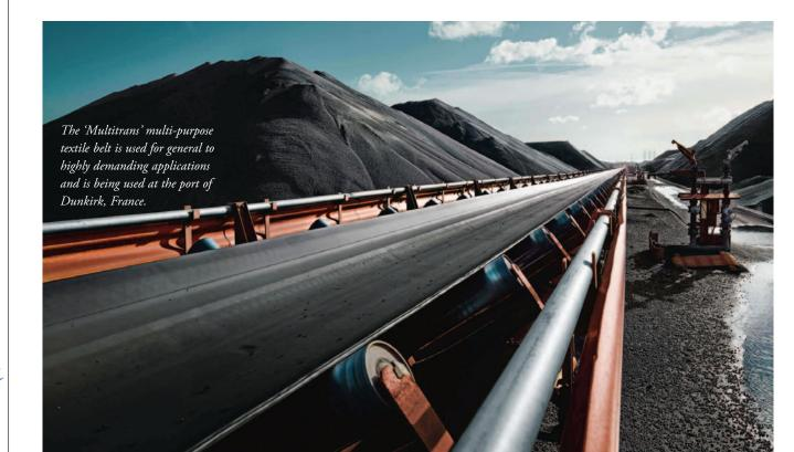
process. Sempertrans successfully implemented the energy-saving belt TransEvo Ultra for surface mining and TransEvo-V for underground coal mining. These belts enable power savings of up to 25%, which is highly recommended in case of long-distance conveyance to reduce energy consumption.
