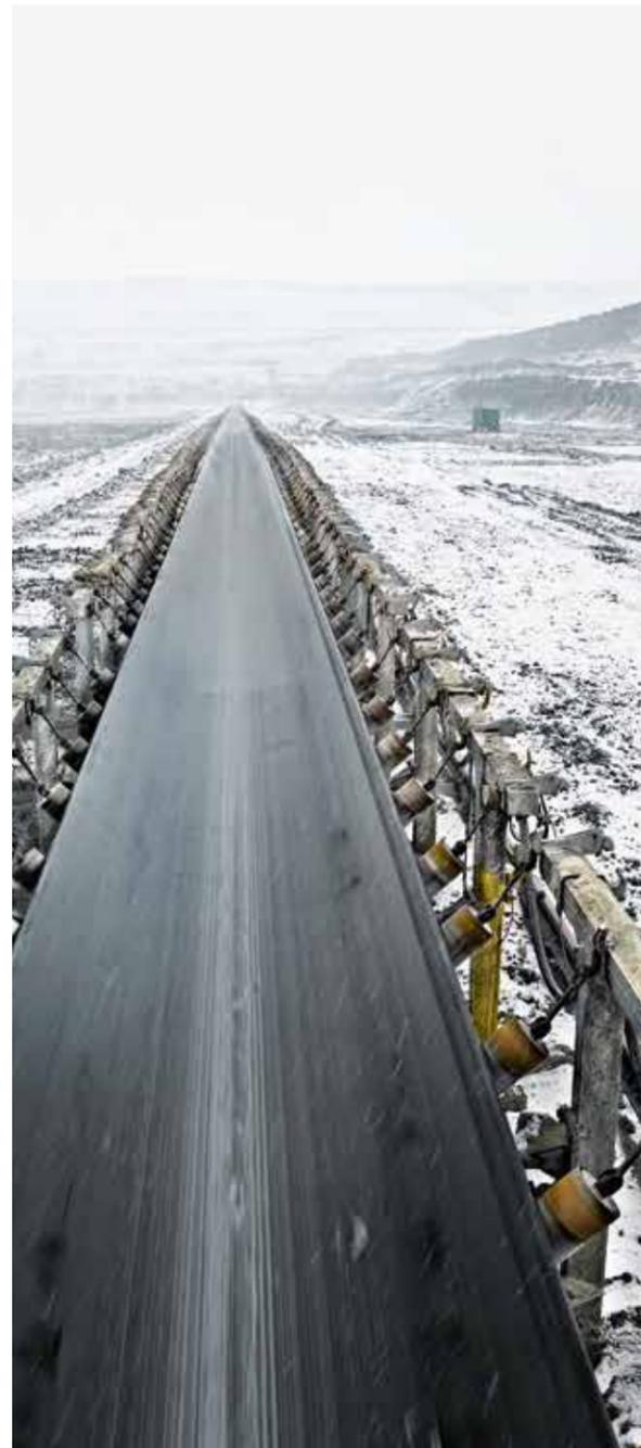
In some regions, conveyor belts are exposed to extremely large temperature ranges. The belt structure can get brittle and be subject to cracks at temperatures below -30 °C.
