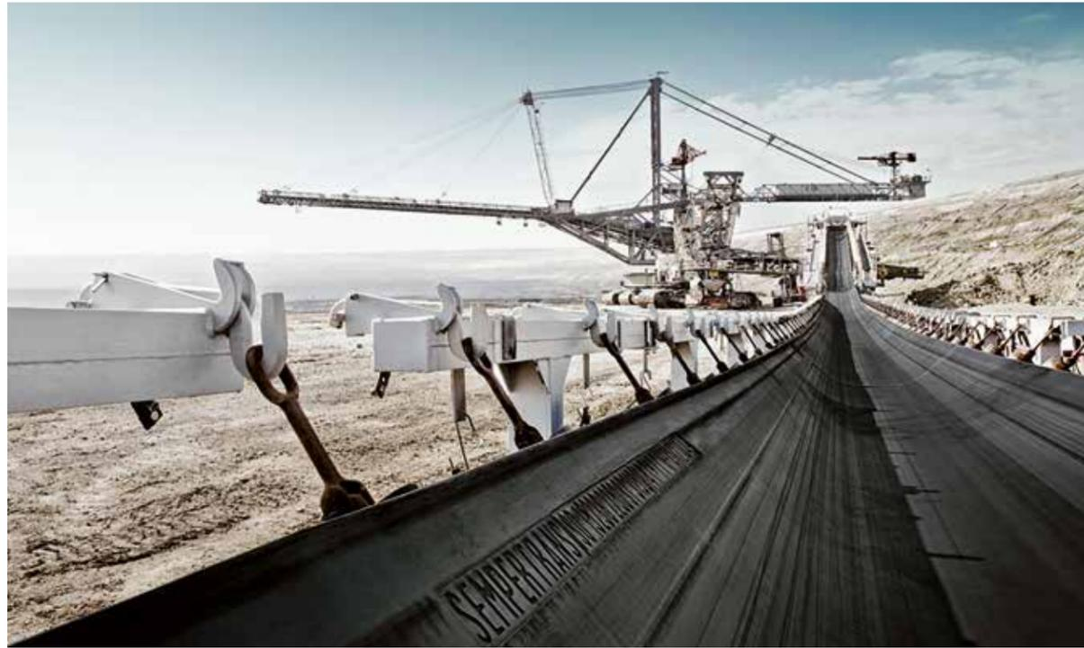
TransEvo covers are based on a special rubber compound which significantly reduces rolling resistance due to indentation losses while the belt is running over the idlers. TransEvo achieves energy savings of up to 25% compared to conventional conveyor belts, proven by both external testing facilities and field tests at several installations at Sempertrans customers' sites.
