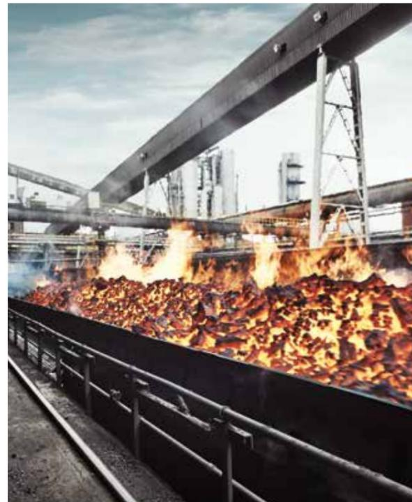
**S:** Flame retardant cover and carcass according to ISO 340, anti-static according to ISO 284. For general use with electrical and fire safety requirements in line with EN 12882 as well as the former German grade S as defined in DIN 22102.
