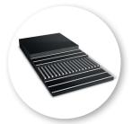
The Translev M has a **full steel carcass design**. Steel cords in longitudinal direction provide high nominal belt strength at low elongation, as well as two layers of steel wefts in cross direction. This construction provides the highest bolt pull-out values combined with the highest possible puncture resistance.
