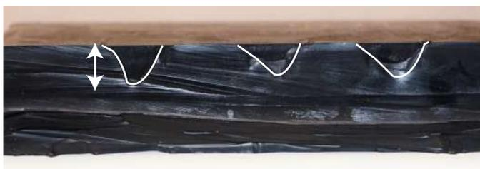
Cross Section of DIN X Cut Depths
