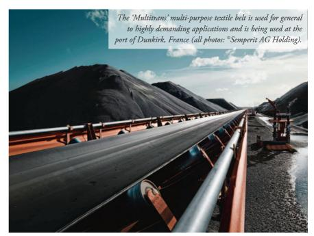
used to transport dry bulk material, like coal, iron ore, cement, sand and gravel, grain but also chemical products, in the mining, steel, cement industry, at ports, but also in other applications like power and heating plants.
